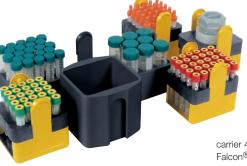
carrier 4522-A with adapters for Falcon<sup>®</sup> tubes, blood collection tubes and bottles
